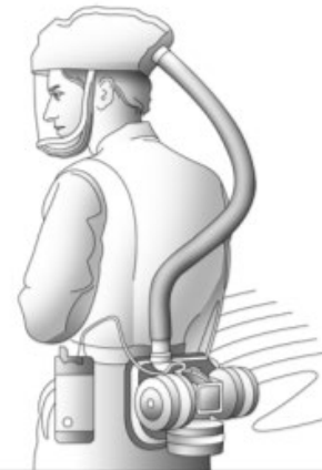
Loose-Fitting Powered Air-Purifying Respirator (PAPR) APF=25
